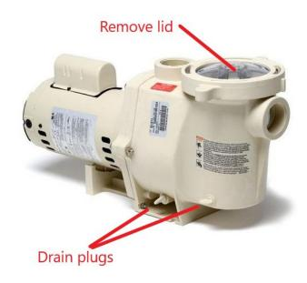
4- Pump winterization- booster pumps. You can either locate and remove the plug on the front of the pump volute, or simply remove the frontside flexible hose and tilt the pump forward to drain the water.
